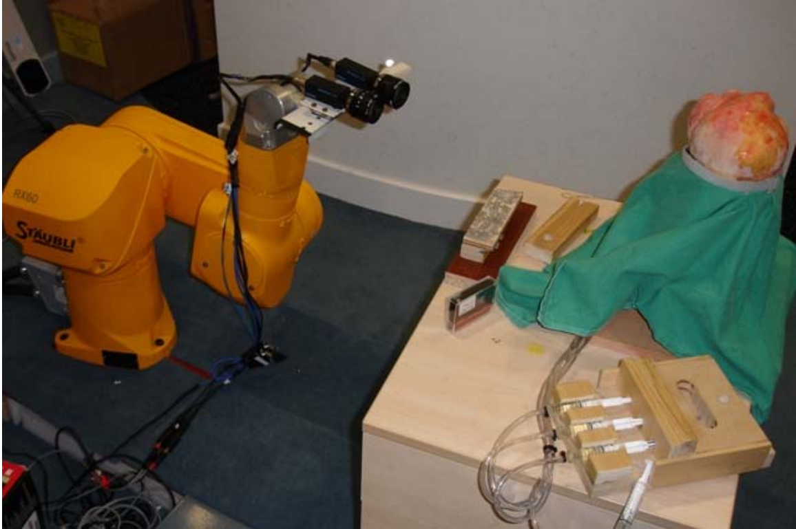
Figure 11. Gaze-contingent robotic system.
